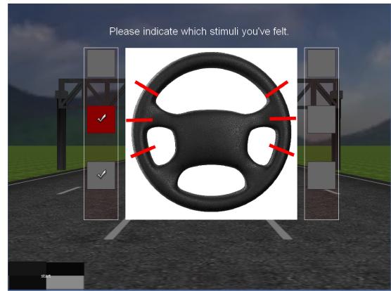
Figure 4. User feedback screen. Each check box corresponds to a solenoid on the steering wheel. Left top to bottom: L1-L3, right: R1-R3.
